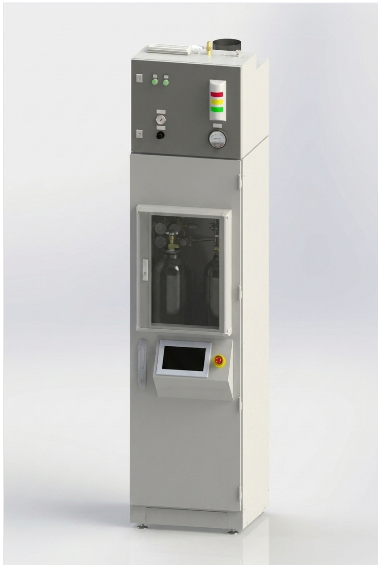
GASPOD cabinet — head with status column, gauges & touch-screen; body with viewing window & EMO button
